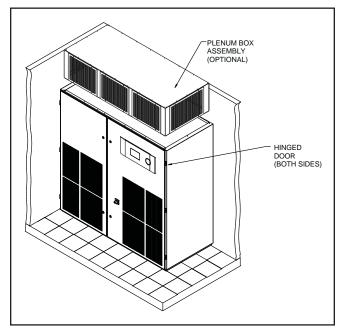
Figure 6- Typical Installation Upflow
