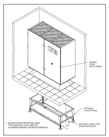
Figure 7- Typical Installation Downflow
