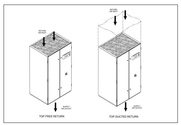
Figure 9- Downflow Configuration Air Patterns
