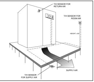
Figure 15- Temperature/Humidity Sensor Location
