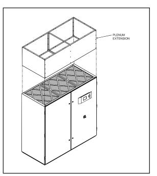
Figure 14- Plenum Installation
