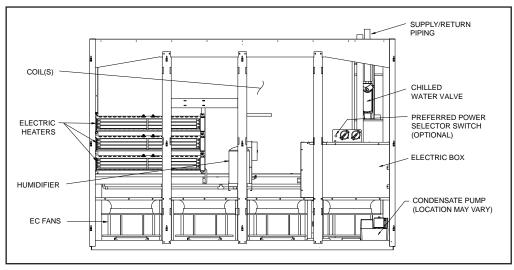
Figure 2- Typical Internal Layout- Downflow (Model CCD-3600-CWE shown for reference)
