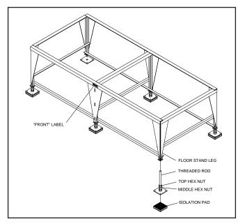
Figure 10- Floor Stand Installation
