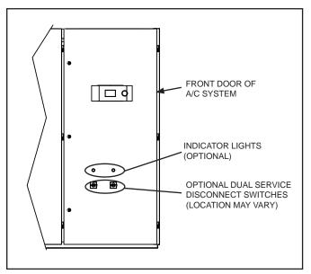
Figure 3- Auto Transfer Disconnect Switches
