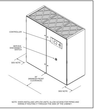
Figure 5- Recommended Installation Clearance
