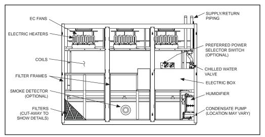
**Figure 1- Typical Internal Layout- Upflow** (Model CCU-2300-CWE shown for reference)
