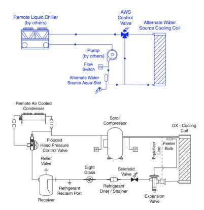
Figure 3. Free Cooling Diagram
