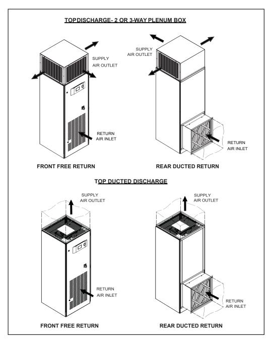
Figure 8. Upflow Configuration Typical Air Patterns
