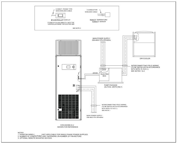
Figure 15. Interconnecting Field Wiring Glycol Systems
