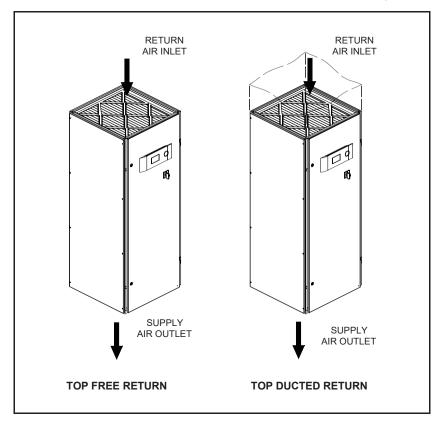
Figure 7. Downflow Configuration Typical Air Patterns
