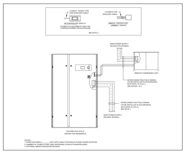
Figure 14. Interconnecting Field Wiring Remote Condensing Unit
