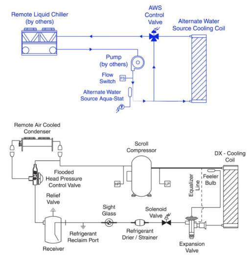
Figure 4. Alternate Water Source Diagram
