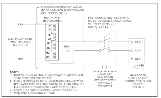
Figure 12. Transformer Schematic
