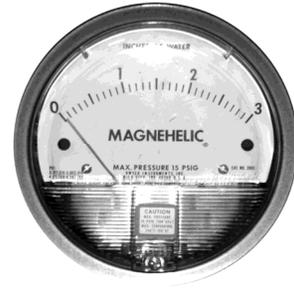
**Figure 7 - Differential Pressure Gauges**
