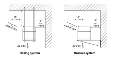
Figure 2. Installation of Humidifier
