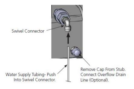
Figure 5. Water Inlet Connector
