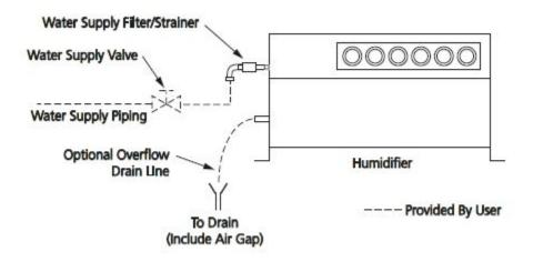
Figure 4. Piping Connections
