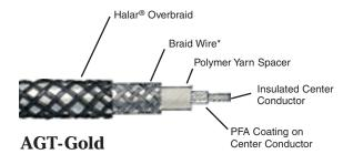
**AGT-Gold** is a wicking cable specially designed for the detection of accumulations at a shallow depth of 1/16 inch of liquid. The cable is chemically resistant and designed to detect water, highly corrosive acid, base and solvent leaks in computer rooms, clean room sub-floors, above ground single wall pipes and equipment applications. This cable requires more drying time than AGW-Gold.
