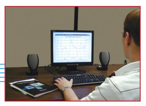
PALCOM<sup>®</sup> software, (for Windows<sup>®</sup> 98/NT/XP) can centrally monitor up to 254 PAL-AT monitoring units. A computer is connected to the PAL-AT units, using either twisted pair wire or modems. The software has the ability to continuously monitor the status and/or remotely operate each PAL-AT.
