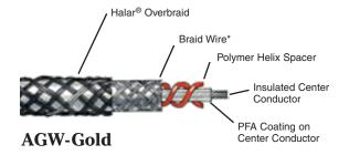
**AGW-Gold** is a quick drying cable, that is chemically resistant and designed to detect highly corrosive liquid leaks, such as acids, bases and solvents. Typical applications are secondary containment pipes, computer rooms, sub-floors of clean rooms and high temperature applications.
