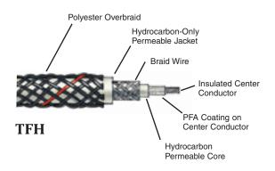
**TFH** is a wicking cable specifically designed to detect only hydrocarbons. This cable may be direct buried to a maximum depth of 20 feet to locate fuel leaks while ignoring the presence of water. This cable is ideal for monitoring single-wall pipes and tanks.
