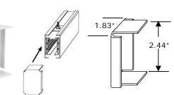
WEIGHT Plate Type For concealed connecting 0.8 lb Plate Type Busway sections. One required. PART NUMBER Wrap Around Type HC-1 For connecting Busway WEIGHT sections on the outside of 0.4 lb Wrap Around the Busway. One required.
