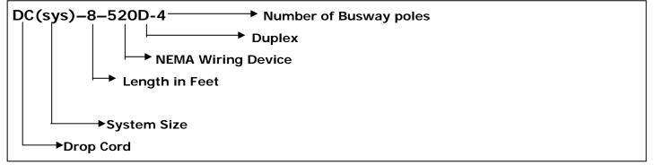
For B225 System, *Circuit Breaker protection* with one 10 ft Drop Cord with NEMA L6-30 Connector and one 10 ft Drop Cord with L5-20 Connector
