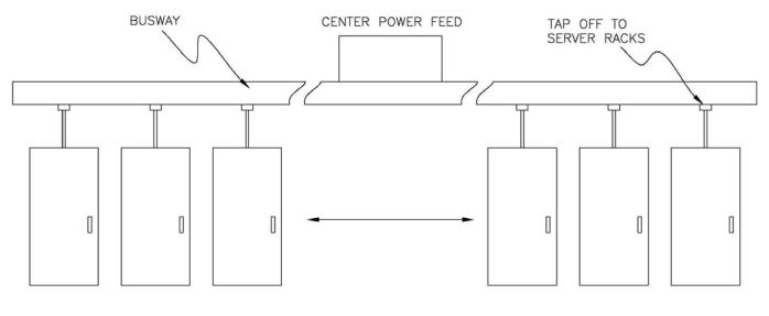
FIGURE 2: BUSWAY APPLICATION WITH DUAL NEUTRAL CENTER FEED
