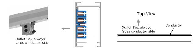
Tee's and Elbow Sections are specified according to desired polarity
