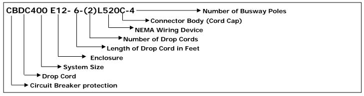
For B400N, a single, 8 ft Drop Cord with 5-20 Duplex, fuse protection
