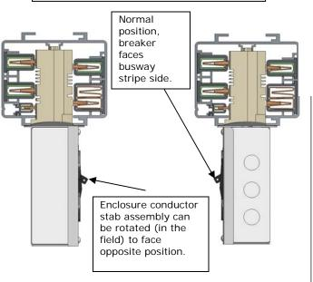
Circuit Breaker Plug-In E12 Enclosure Applications with Receptacle Receptacleplications
