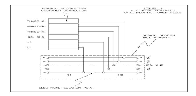
Refer again to Figure 2. The system is capable of a total of 225 amps per phase across the entire system length. More importantly, the system is capable of 225 amps neutral current to the left of the power feed, and another 225 amps neutral current to the right of the power feed. The end result is that with a single power feed point and therefore a single conduit home run, the busway system provides 225 amps per phase and 450 amps neutral capacity.
