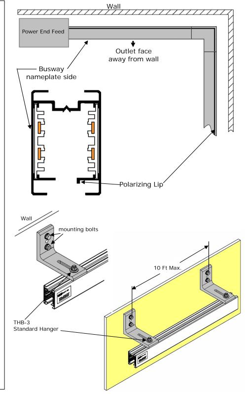
Polarizing lip orientation is vital to the proper installation of STARLINE Track Busway. The polarization lip should face the wall when using fuse protected outlet boxes or drop cord plug-in units. This insures that outlets will always face away from the wall. When using circuit breaker or fused disconnect plug-in units, the polarization lip should face *away* from the wall. The polarization lip is always located on the opposite of the Busway name plate.
