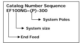
**POWER FEED UNITS** Supplying power to End of Busway
