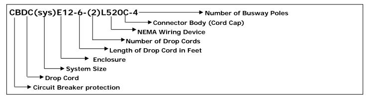
For B100N, a single, 8 ft Drop Cord with 5-20 Duplex, fuse protection
