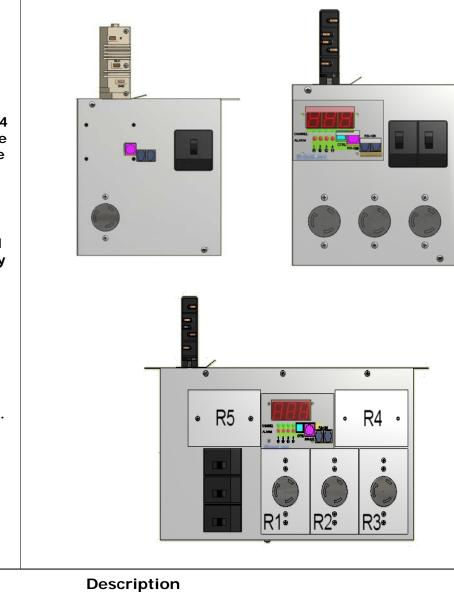
**Circuit Breaker Unit with Installed Current Monitor**
