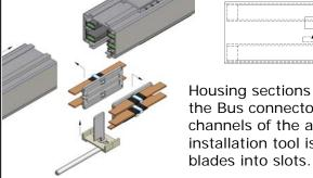
Tool Force Housing sections are joined by inserting the Bus connector which fits into the channels of the adjoining section. The installation tool is then rotated to force
